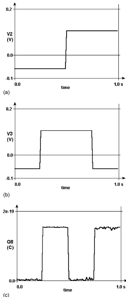
Fig. 8. Operation of the single-electron CCN gate as a XOR gate. (a) Time variation of the input voltage  $V_2$ , (b) time variation of the input voltage  $V_3$  and (c) time variation of the charge in the output island  $N_8$ .
