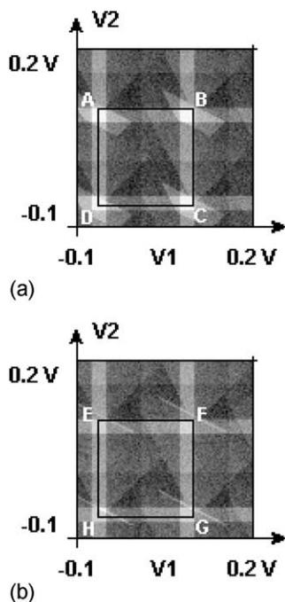
Fig. 7. Stability plots of the single-electron CCN gate,  $V_2$  versus  $V_1$ , (a)  $V_3$  is constant and equal to  $-60$  mV and (b)  $V_3$  is constant and equal to  $105$  mV.
