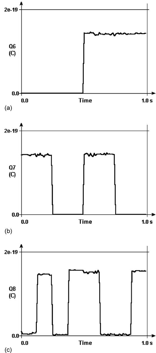
Fig. 4. Output signals of the CCN gate. (a) Time variation of the charge in the island  $N6$ , (b) time variation of the charge in the island  $N7$ , and (c) time variation of the charge in the island  $N8$ .
