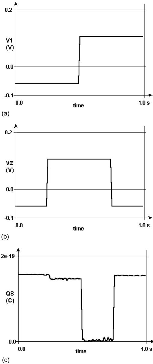
Fig. 10. Operation of the single-electron CCN gate as a NAND gate. (a) Time variation of the input voltage  $V_1$ , (b) time variation of the input voltage  $V_2$  and (c) time variation of the charge in the output island  $N_8$ .
