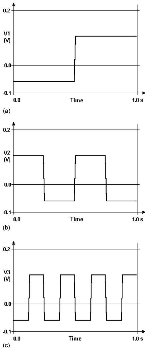
Fig. 3. Input voltages of the CCN gate. (a) Time variation of voltage  $V1$ , (b) time variation of voltage  $V2$  and (c) time variation of voltage  $V3$ .
