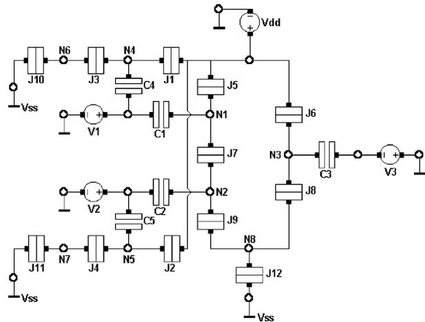
Fig. 2. The circuit of the single-electron CCN gate.
