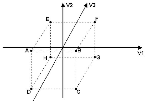
Fig. 6. The Cartesian space spanned by the three input voltages, and the three-dimensional stability plot of the gate with the eight operating points A–H.
