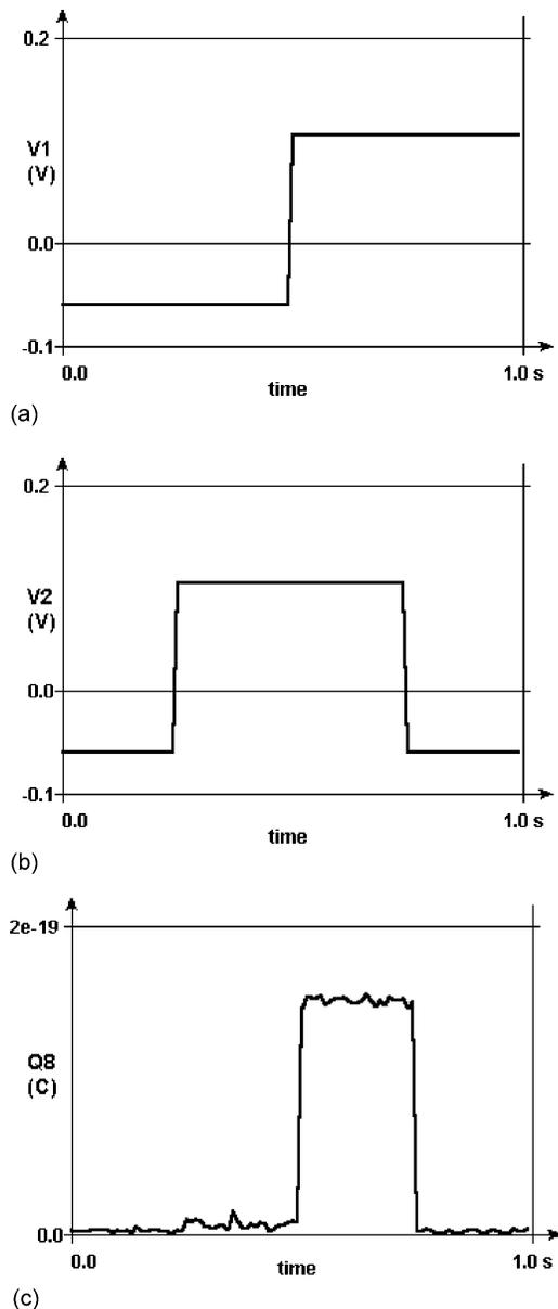
Fig. 9. Operation of the single-electron CCN gate as an AND gate. (a) Time variation of the input voltage  $V_1$ , (b) time variation of the input voltage  $V_2$  and (c) time variation of the charge in the output island  $N_8$ .
