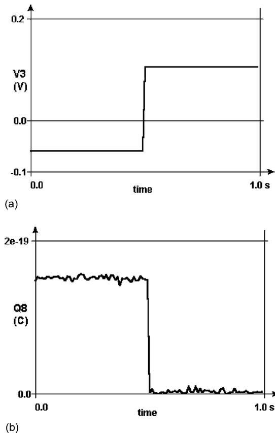
Fig. 11. Operation of the single-electron CCN gate as a NOT gate. (a) Time variation of the input voltage  $V3$  and (b) time variation of the charge in the output island  $N8$ .
